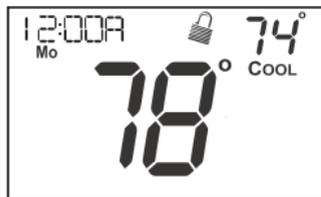
To unlock the keypad, press and hold the **MODE** button. While holding the **MODE** button, press the **WARMER** and **COOLER** buttons together, the
